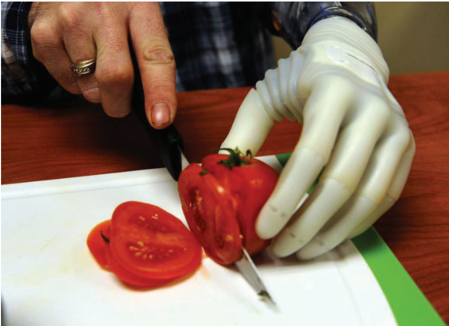
Matt Razink has begun the orientation and training for his new battery-powered artificial hand with an opposable thumb.
